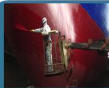
Hull Coating (Ultra-Fine Self-Polishing Paint)
